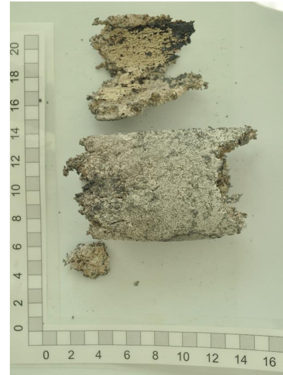
Fig. 2: Clogging at the submerged entry nozzle (SEN)
