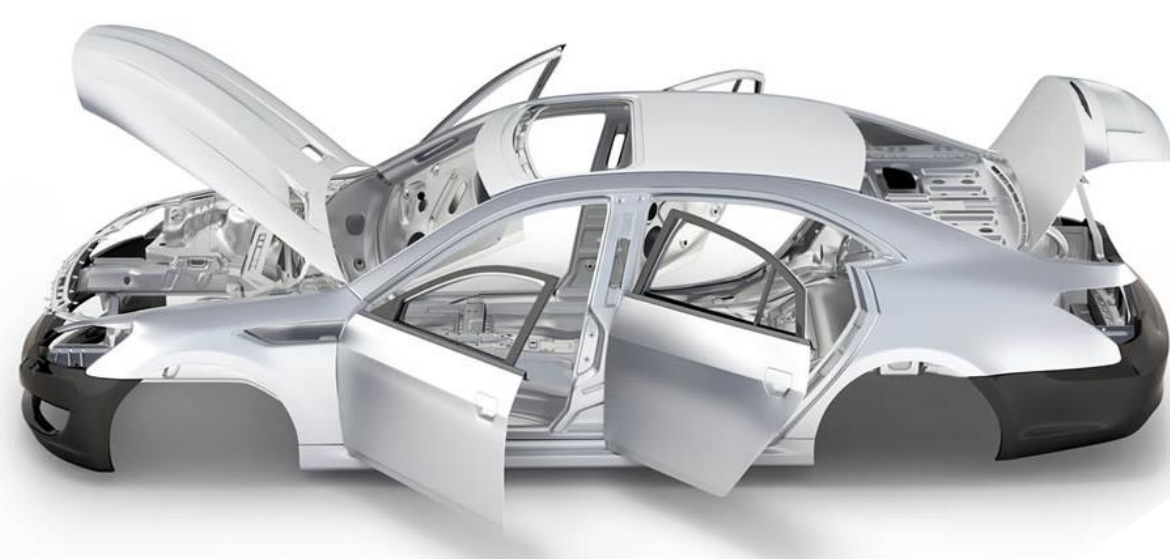
Fig. 3: Automobile panels as an example for the use of Ti-ULC steel. [2]
