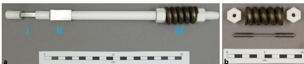
The load was applied to the CLT specimen with a spring made of a cobalt-base alloy and ceramic nuts (Fig. 2b), the latter ensuring electronic decoupling of the specimen from the more noble spring. The specimens were connected with PTFE parts.
